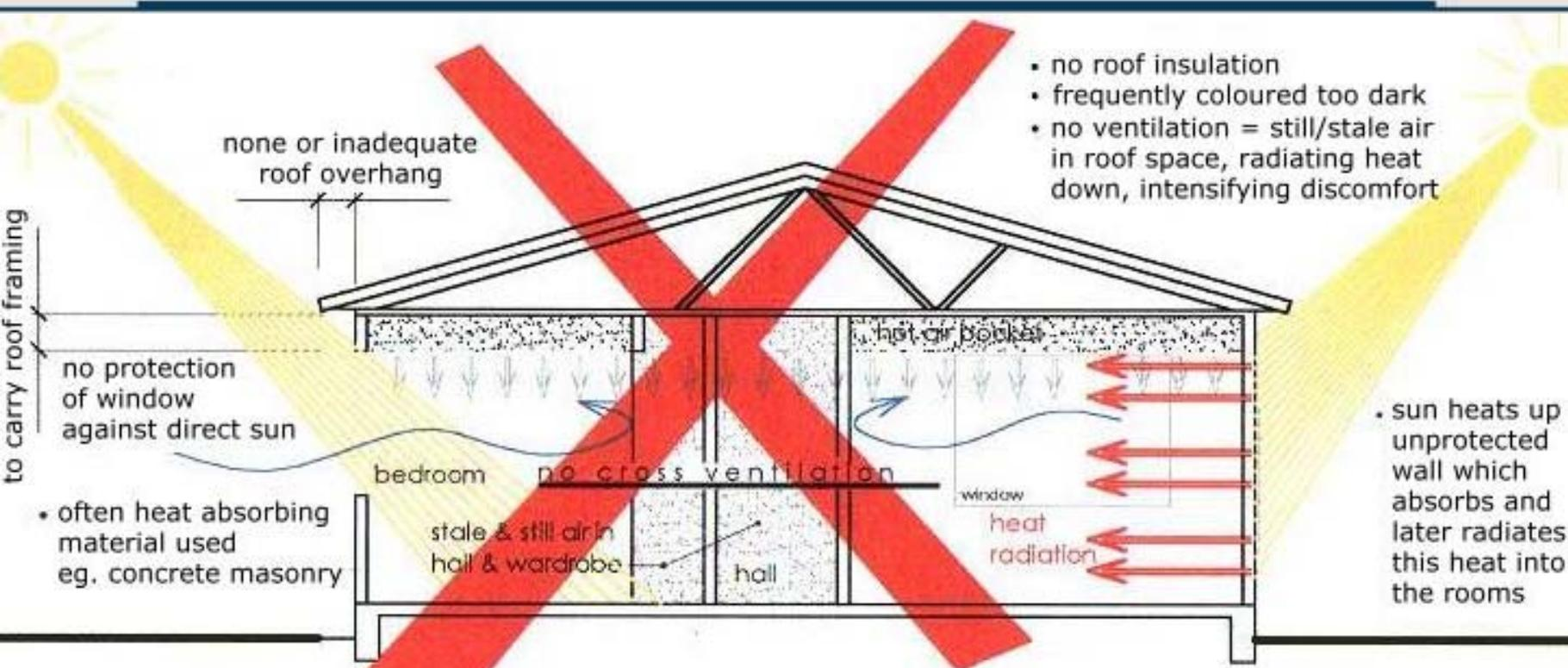
conventional cross section & construction method (roof trusses)
