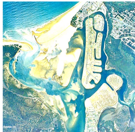
October 1978, showing construction of the spit and changes underway in the river mouth
